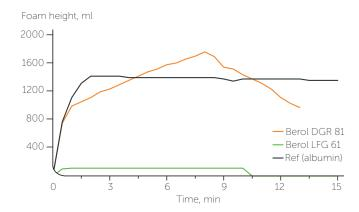
Foaming profile of Berol DGR 81 and Berol LFG 61 when tested in the circulation method. Albumin was used as a foaming agent. The graph shows that Berol LFG 61 provides anti-foaming properties in this system at 0.033%.
