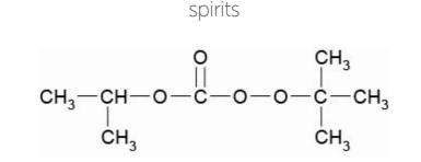
Trigonox BPIC-C75 is an initiator (75% active ingredient in odorless mineral spirits) for (co)polymerization of acrylates and methacrylates.
