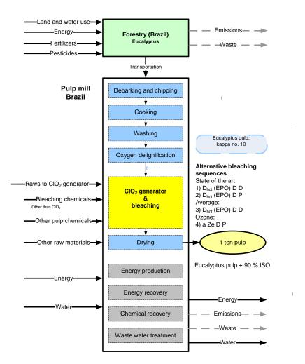
Figure 2: The system studied. In the Chemical Island scenario, the sodium chlorate plant is also located at the pulp mill site.
