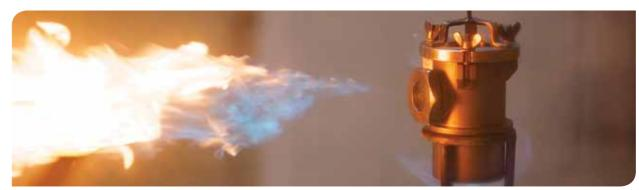
Safety testing to determine the sensitiveness of peroxides to the effect of heat under confinement
