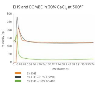
Fig.4 Breaking effect of VES GEL through EGMBE as a mutual solvent post-flush
