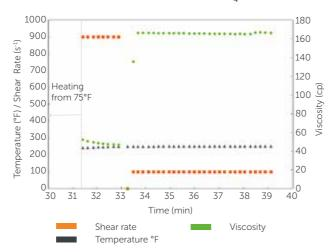
Fig.6 Example of viscoelastic properties of VES fluids (6% VES in  $\rm NH_4Cl$  brine)
