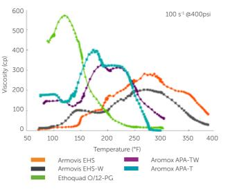
Fig. 1 Viscosity vs. Temperature functionality of Nouryon VES portfolio
