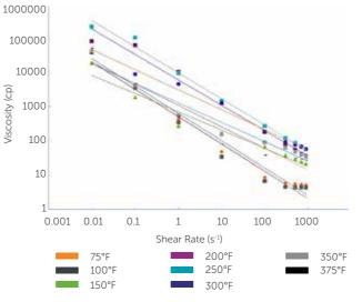
Fig. 5 Example of shear-thinning viscosity of VES fluids
