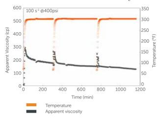
Fig.2 Thermal Stability of Armovis EHS in depleted acid (20% HCl -> 30% CaCl, brine) at 300°F
