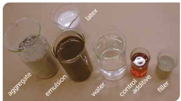
Slurry surfacing mix design components.
