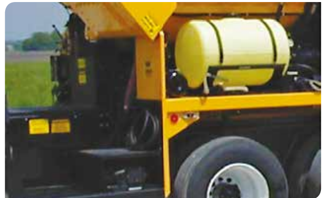
Additive tank on the paver. Additive is used to extend the mix time in hot weather.
