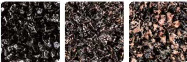
Visual estimation of aggregate surface area covered with bitumen.
