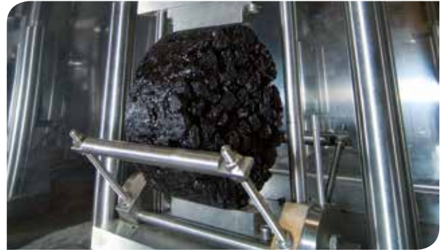
The Nottingham asphalttester can be configured for different type of tests.
