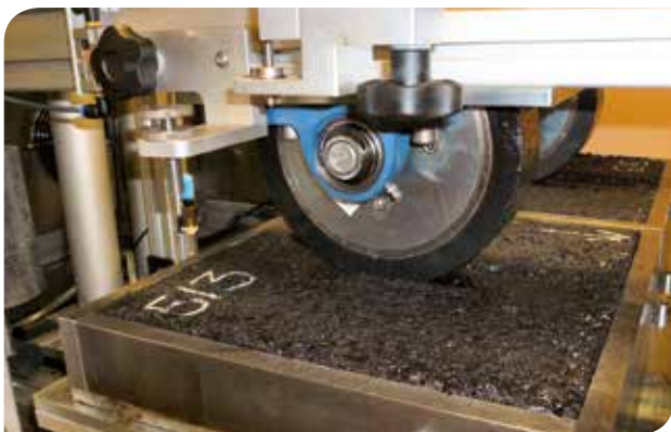
Typical test equipment for measurement of slabs (KVD laboratory, Norway)..
