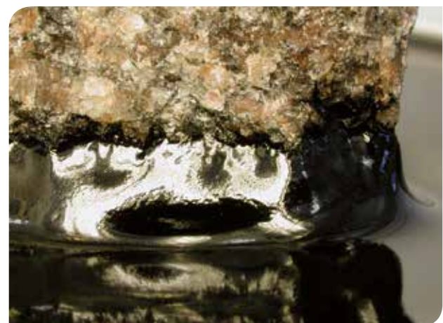
The use of untreated bitumen may result in stripping leading to detachment of the bitumen film from the aggregate surface.
