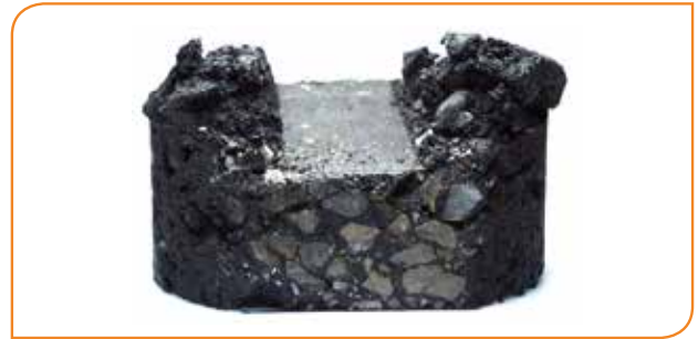
Wheel Track test results from SBUF-report 0071
