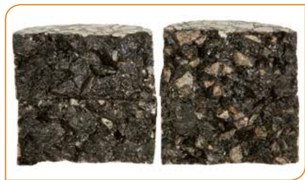
Effect of adhesion promoter on soaked specimens, sample to the left contains adhesion promoter.
