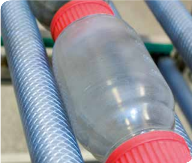
Bottles containing bitumen covered single sized aggregate chippings and water in the rolling device.
