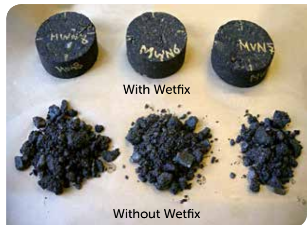
Test results with and without adhesion promoter in foam mixes.
